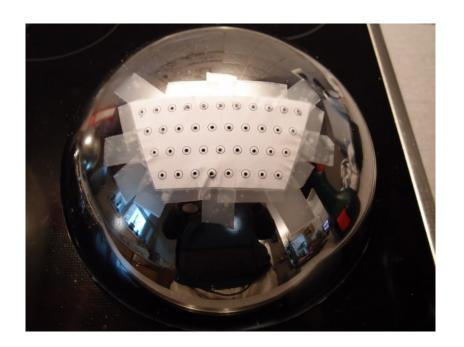
From the back drill all holes with 5mm dia drill
