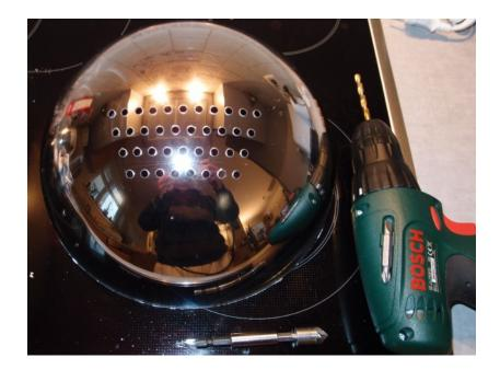
I used a spanner and 2 wires to force a egg shape. wires go through the 2 extra holes which are below the ones for the elastic. adjust as you want it. Force it a little bit more because after tempering it will spring back a bit.
