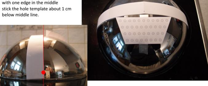
From the front drill 2mm dia. holes in the center of each hole Don't drill too fast, don't push hard! use new/sharp drill I used a battery hand drill
