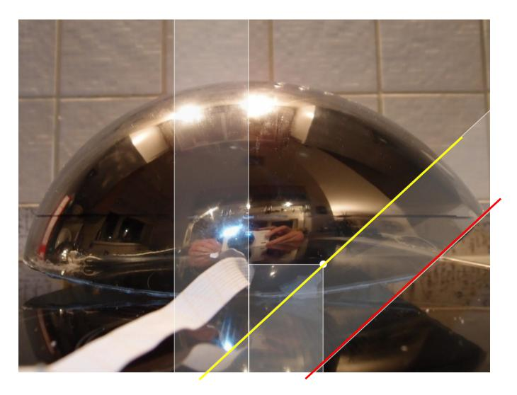
Place Ruler with one edge touching lower hole at about 45°, trace a line and cut of lower section with the dremel this is so the neck has more freedom.
